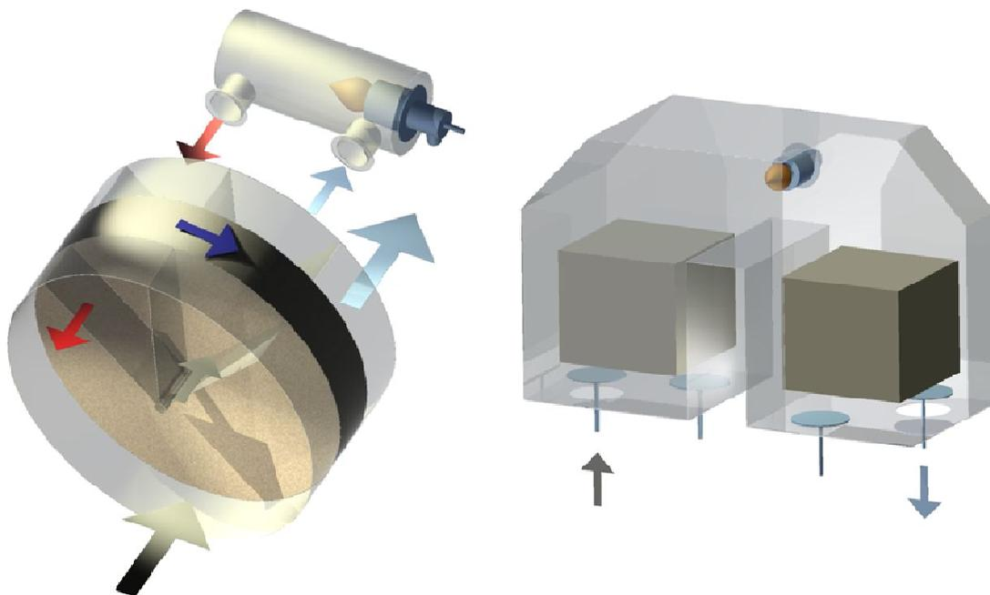
Waste air (cold stream) passes through the rotor where, in the first part, adsorption of VOC takes place on the hydrophobic zeolite adsorbent, followed by displacement of VOC into a small heated air stream. The concentrate is then treated in a suitably chosen regenerative thermal oxidation (RTO) system. The rotor therefore ensures increasing concentrations of
